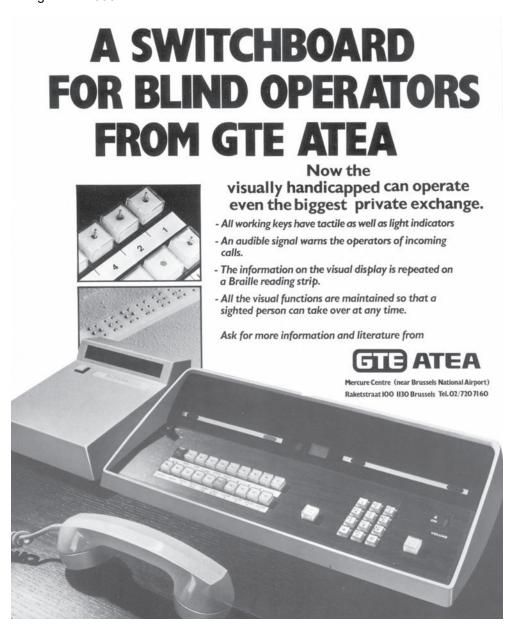
ATEA, the Belgian telecom company I worked for, was, from 1926 to 1986, a subsidiary of the American company Automatic Electric of Chicago. Where originally American technology (such as Strowger) was used to design European products, this changed in the 1970s. Given the ever-increasing complexity of telephony, the decision was made to take over American telephone exchanges as a whole and adapt them to international standards.
