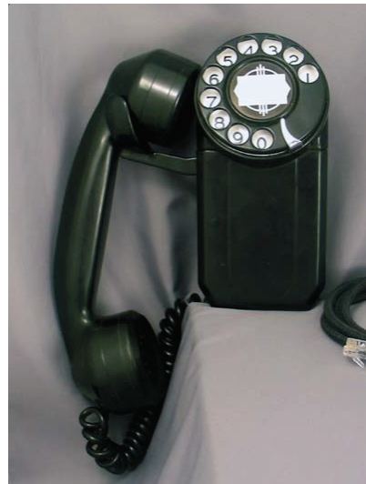
Figure 16: Automatic Electric Model 43 Spacemaker with zinc alloy body
