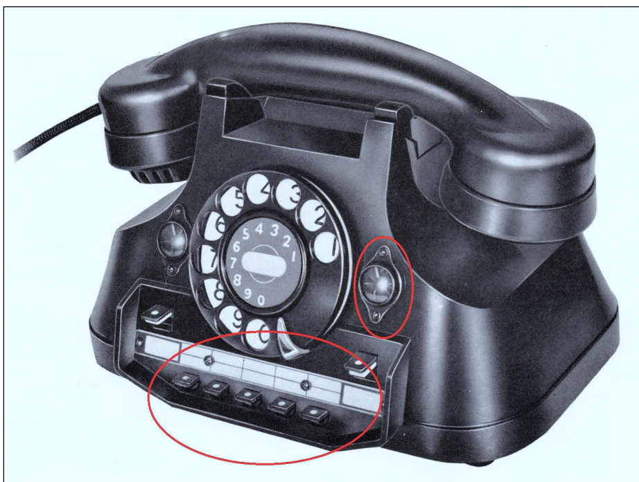
Fig. 5 keys and visual indicator from a 1950 key system
