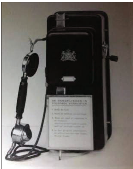
Fig. 7 - Berliner (+/-1920) Dutch PTT payphone (courtesy Jan Jansen, NL). The incoming coin activated a gong, which was acoustical forwarded to the operator via a small microphone.
