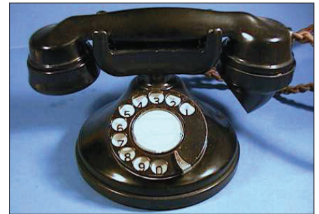
Fig. 3 The ATM Strowgerphone ATM made basically the same phone as AE, The major difference was the BPO type 164 handset.
