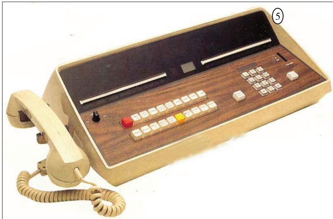
1976 attendants console (GTD120/1000)c Housing: plastic Technology: electronic
