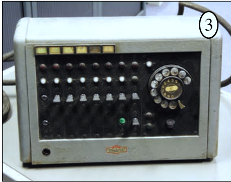
1950's attendants console Housing: metal Technology: electro-mechanical
