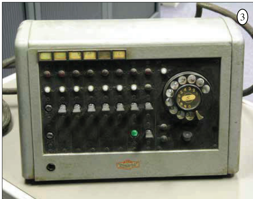
1950's attendants console Housing: metal Technology: electro-mechanical
