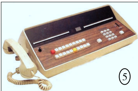
1976 attendants console (GTD120/1000)c Housing: plastic Technology: electronic
