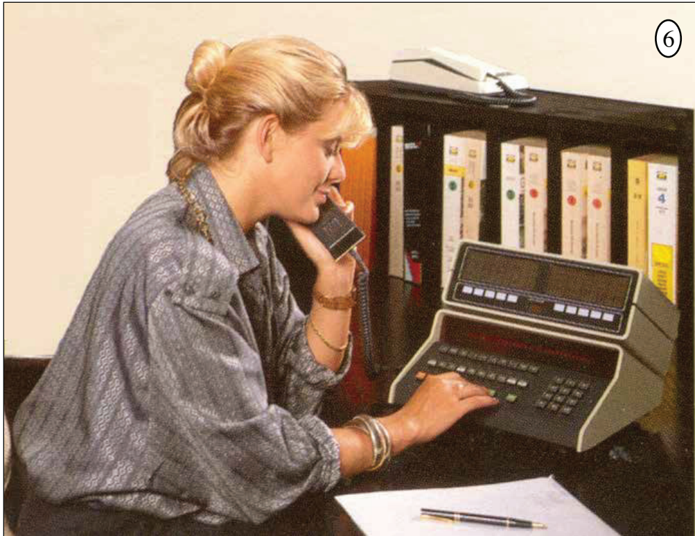
1983 attendants console (OMNI PACET) Housing: metal/plastic Technology: electronic, software controlled via data-link
